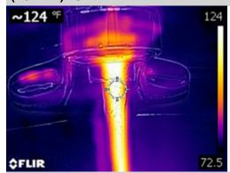
The hot water temperature for the home was noted to be too high. The recommended temperature to prevent personal injury and burns is 120 degrees F. The elevated temperature could indicate a malfunction or problems with the water heating unit. A licensed plumbing contractor should be consulted to evaluate the system to ensure that the water heating unit is operating correctly and within a safe temperature range.
